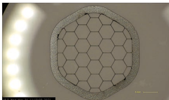
Figure 2: A niobium mesh micromachined using a 1033nm fs laser to provide a support for a thin film filter.
