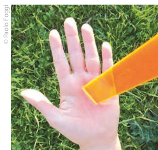
A piece of LSC material, showing increased brightness at the hand.
