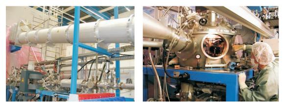
Beam transport structure (left) and target chamber (right) used for combined heavy ion and laser experiments.
