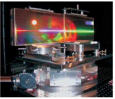
A photograph of the Phased Array grating system developed at the FSU as part of the OTTER programme.
