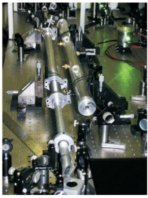
Hollow-fiber experimental setup for the compression of high-energy laser pulses down to sub-5-fs duration. The gas-filled capillary is contained in the metallic tube on the left-hand side of the photograph.
