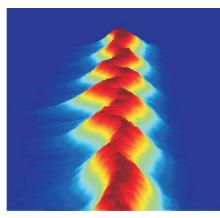
Three-dimensional plot of the evolution of the experimental photoelectron spectrum (horizontal axis) as a function of temporal delay (vertical axis) between the attosecond and the infrared 5-fs pulses. From this trace it was possible to retrieve a 130-as duration for the isolated attosecond XUV pulses.
