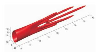
Computer simulation of an intense, ultra-short pulse propagating through a transparent medium indicating the onset of filamentation and self focussing leading to catastrophic damage.
