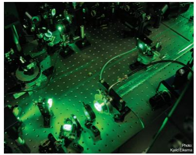
Optical Parametric Amplifier used within the FOSCIL JRA at LCVU.
