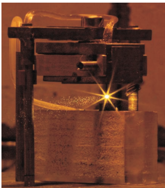
Femtosecond pulses focussed into a water jet for x-ray fs-pulse generation.
