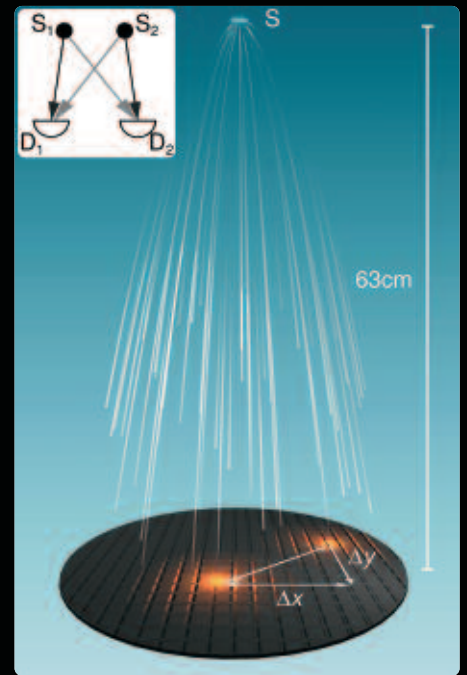
Figure 2. A cold cloud of helium atoms is released from the magnetic trap (Fig. 1), expands and falls under the influence of gravity on a time-resolved and position-sensitive detector that detects single atoms. The inset shows how bunching and antibunching occur when two possible paths interfere: S_1 and S_2 refer to two source points and D_1 and D_2 to two detection points. For bosons the two amplitudes \langle D_1 | S_1 \rangle \langle D_2 | S_2 \rangle and \langle D_1 | S_2 \rangle \langle D_2 | S_1 \rangle have to be added, which yields a factor of 2 in the joint detection probability if the two amplitudes have the same phase (within the coherence volume). For fermions the two amplitudes must be subtracted, yielding a zero probability for the joint detection in the same coherence volume.
