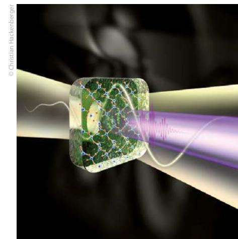
Ultrafast lasers drive the motion of electrons inside silicon dioxide to generate extreme ultraviolet radiation.
