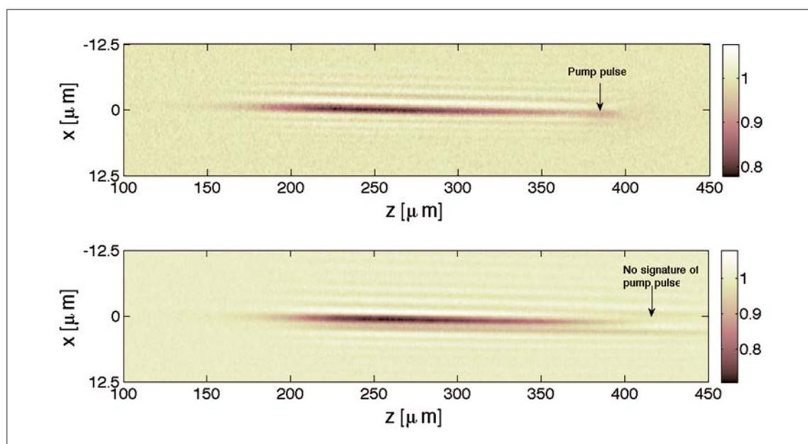
Figure 1: By carefully tuning the probe pulse at the anti-stokes wavelength of the pump pulse, it is possible to detect the pump pulse as an absorption feature of the shadowgram, thanks to an inverse Raman scattering process. The effect is evident from the comparison of the shadowgrams for probe at the anti-stokes (top) and pump (bottom) wavelength. In the latter image the signature of the pump pulse is absent (adapted from Minardi et al. 2014).
