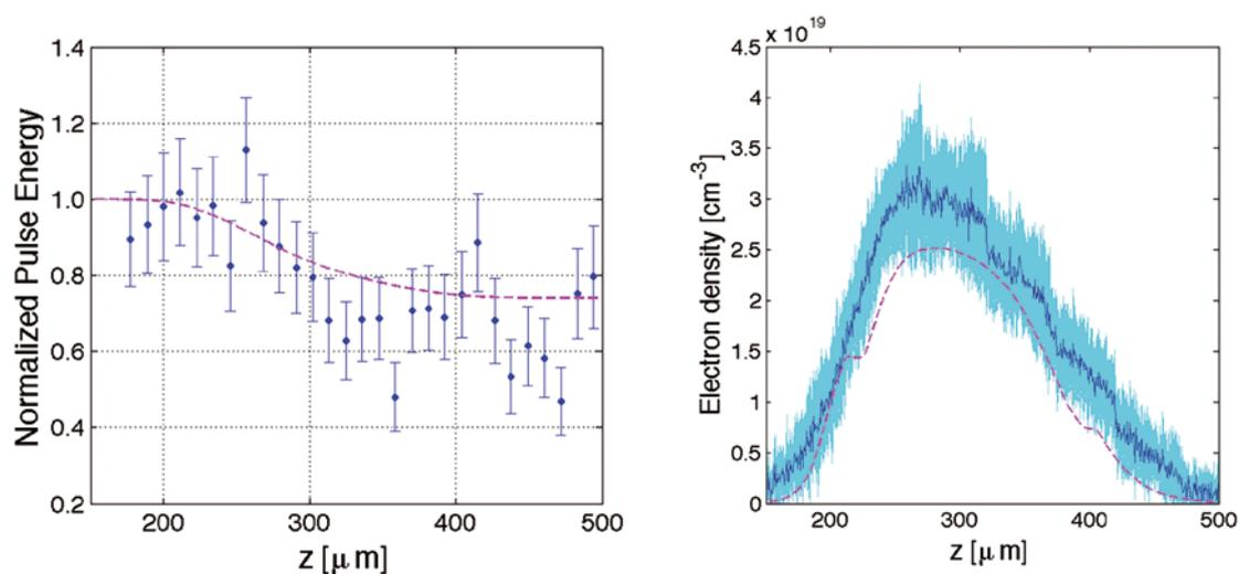
Figure 2: Comparison of experiment with simulation data. Left: the normalized energy content of the pump wave packet as a function of the propagation length. Dots: experimental data. Broken line: numerical simulation. Right: density distribution of the solvated electrons along the propagation coordinate. Blue line: experimental estimate with error (pale blue area). Broken line: numerical simulation (adapted from Minardi et al. 2014).
