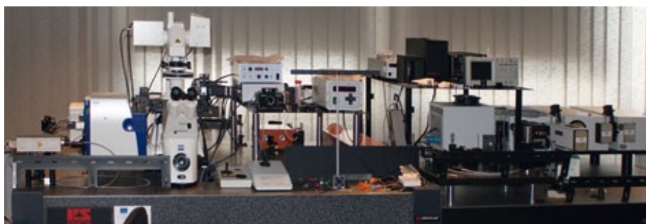
Multi-spectral fluorescence lifetime imaging microscopy setup with non-linear excitation developed at ILC.
