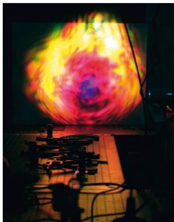
White-light continuum generated by a high-power femtosecond laser.
