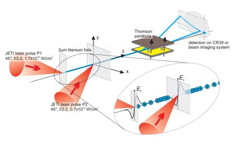
Fig. 1: Sketch of the experimental setup for staged ion acceleration
