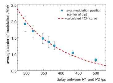
Fig. 3: Central energy of modulated part of the proton spectrum as a function of the delay (left) and generation of a free-standing, quasi-monoenergetic peak in the spectrum using the staged acceleration scheme.
