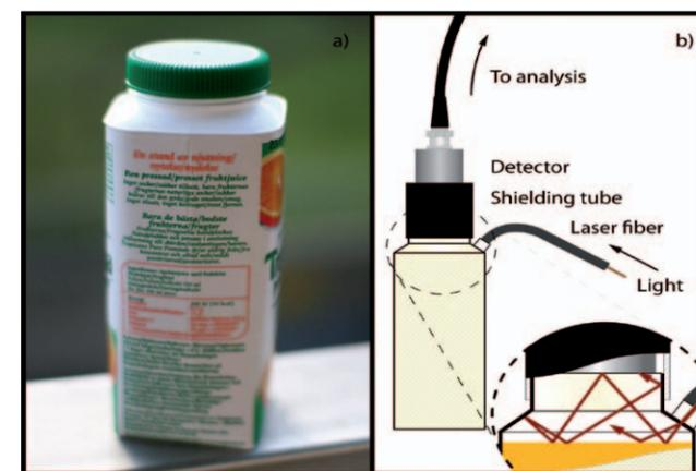
Packaged food quality monitoring by laser spectroscopy: A sample of the orange juice packages studied (left), illustration of the detection geometry (right).
