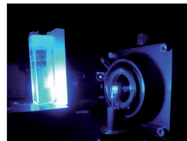
Time-resolved Raman spectroscopy setup; a two layer sample is excited with a 3-ps frequency-doubled Ti:sapphire laser at 460 nm; Raman photons are detected in a backscatter geometry. Photo: Maria Lopez-Lopez
