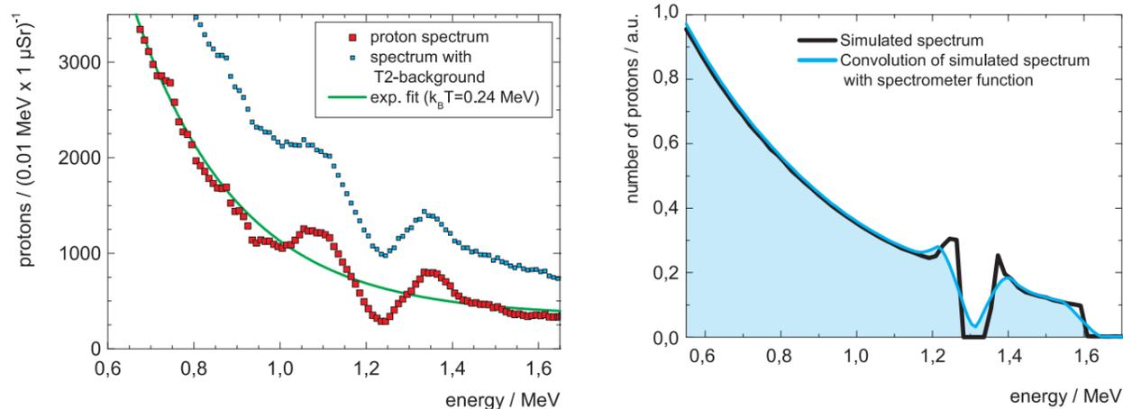
Fig. 2: Measured (left) and simulated (right) proton spectrum after double-stage acceleration.
