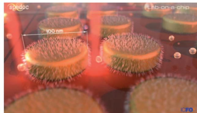
Detection of HSP molecules at the surface of gold nanosensors. © ICFO. Picture by Digivision
