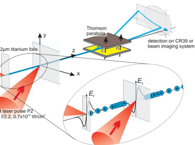
Fig. 1: Sketch of the experimental setup for staged ion acceleration
