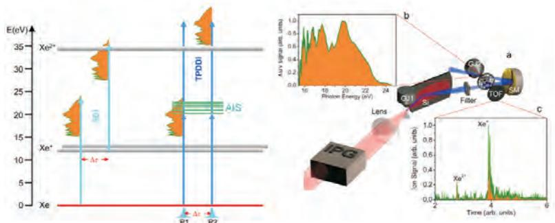
Left: Sequential vs direct double ionization scheme. Right: Experimental set-up (a); the broadband XUV continuum spectrum (b); and the Xe ion mass spectra (c).
