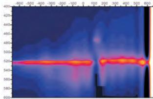
Fig. 1: SFG-XFROG trace obtained with a compressed 1053 nm pulses as probe.
