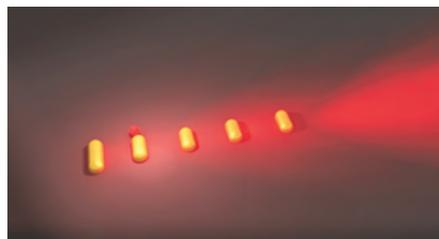
Artist impression of the directional emission of the Yagi-Uda antenna driven by a single luminescent quantum dot. © ICFO
