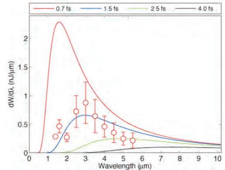
Measured CTR spectra. The continuous lines corresponds to theoretical spectra for the case of gaussian bunches for different duration (from O. Lundh et al., Nature Physics 7 (2011)).
