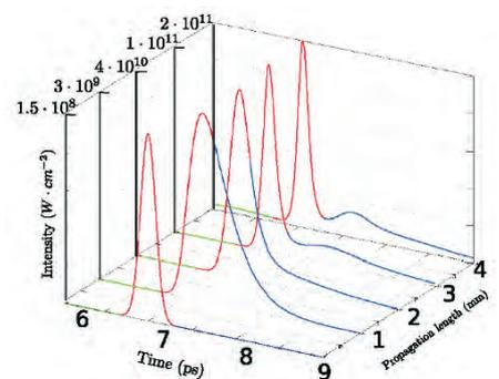
Fig. 2: Pulse shape variation along the plasma amplifier. In green is displayed the ASE, in red the seed and in blue the coherent wake generated by the seed.
