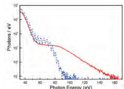
High-order harmonic spectra (number of photons) generated in argon by VIS pulses (dashed curve) and two-color pulses at zero delay (solid curve).
