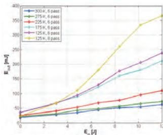
Fig. 2: Temperature dependent output energy versus diode pump energy for the Yb:CaF<sub>2</sub> amplifier seeded with a 57mJ/6ns long pulse.
