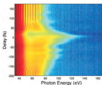
Sequence of harmonic spectra generated in Argon as a function of the delay between the two-color pulses (logarithmic color map).
