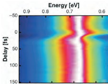
Fig. 2: The measured time dependence of normalized charge transfer resonance (positive delays correspond to times after the pump pulse) showing an oscillation in the peak position at 25 THz.
