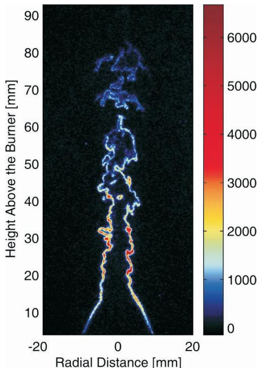
Visualisation of CH in a turbulent flame
