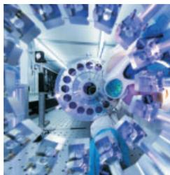
Multi-mirror set-up of a laser amplifier at MBI.
