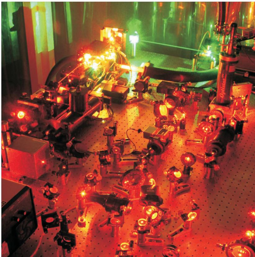
**Fig 3:** Dye laser system frequency stabilized to a line width of 1 kHz. Instead of being locked to a cavity the laser is frequency stabilized against a spectral hole in a Pr doped  $\text{Y}_2\text{SiO}_5$  crystal. (Photo: Tomas Svensson)
