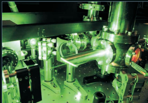
50W Ti:Sapphire system of the Attoscience and Ultrafast Optics group at ICFO
