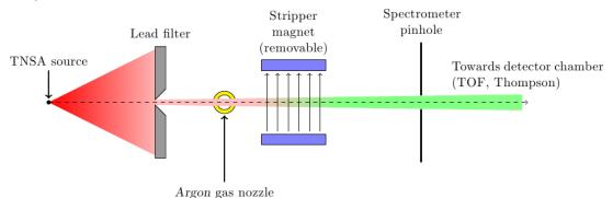
Secondary objective: produce and characterize a beam of accelerated neutral atoms by neutralising the laser accelerated positive charge in an Argon gas jet.
