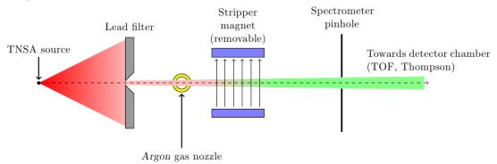
Secondary objective: produce and characterize a beam of accelerated neutral atoms by neutralising the laser accelerated positive charge in an Argon gas jet.
