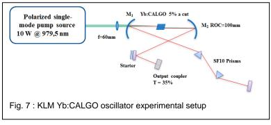
$M_2$ ) in a standard X-fold cavity configuration. To compensate astigmatism due to the Brewster-angle incidence, these mirrors are tilted with an angle of 8°. On one side, the cavity is delimited by a high reflection (HR) mirror and closed on the other side by a 35% outputcoupler (OC). A pair of SF10 prisms separated by a distance
