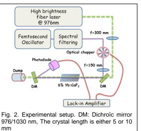
Figure 2 displays the dependence of the gain on the absorbed pump power for 6%Yb:CaF2 5-mm and 10-mm long crystals. The seed, with a spectral width of 2 nm FWHM is centered
