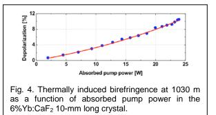
study we have determined that although isotropic, Yb:CaF2 crystal have to be cut along the [111] axis to prevent or limit significantly stress induced birefringence.
