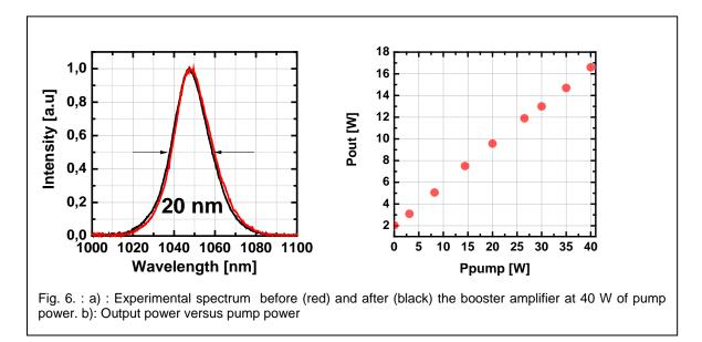
At 40 W of pump power, a depolarization under 1 % is measured and no deleterious thermal effects on beam quality have been observed. These performances are in good agreement with our simulations. The latter reveals very encouraging power and energy scaling.
