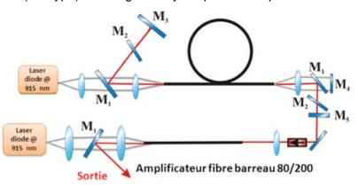
multimode (as compared to operation at 1030 nm). Therefore this configuration is operated below 40 W for an optimal beam quality efficiently used for optical pumping of Yb-doped crystals. The efficiency curve and spectrum is given below.
