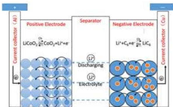
Figure 1 Battery components
