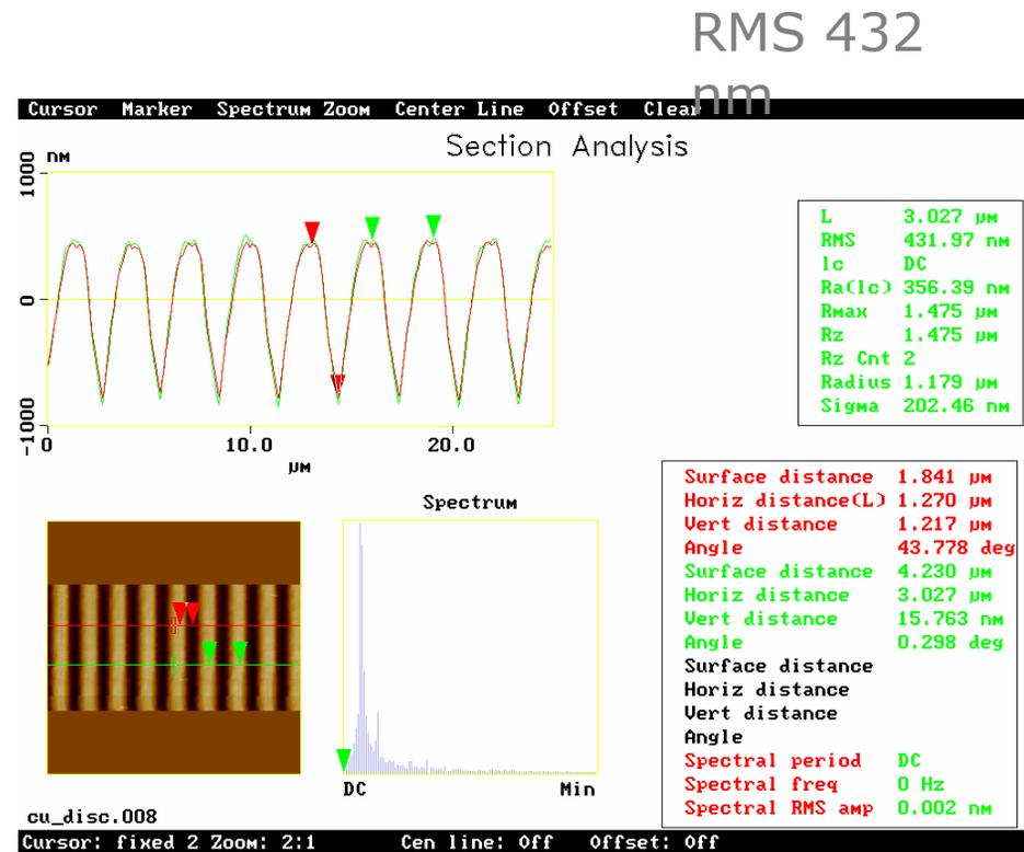
AFM analysis of sinusoidal pattern
