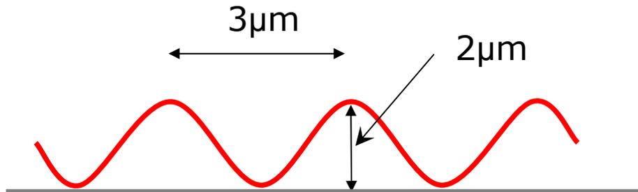
A sinusoidal pattern extending from the edge of an Oxygen-Free High Conductivity Copper disk 13mm inwards.
