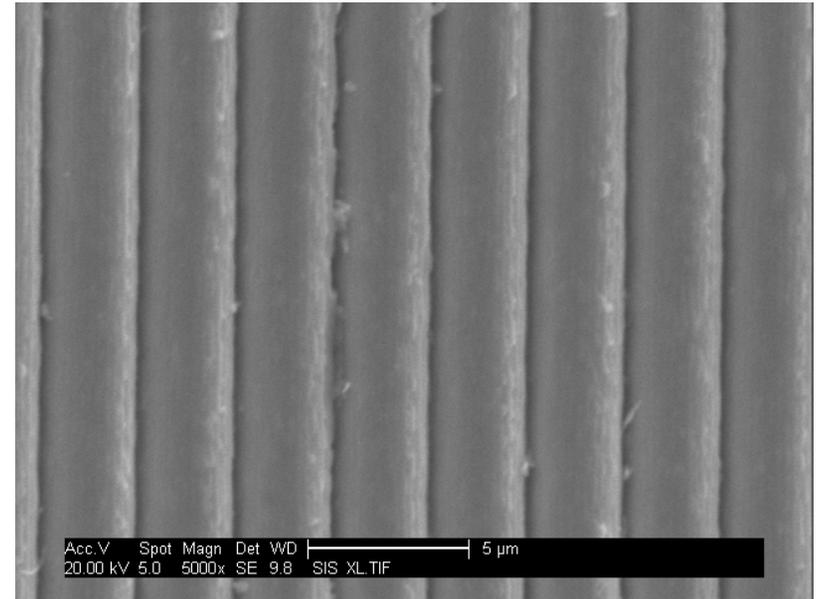
ESEM micrograph of diamond tool showing 'chipping' and wear of the tool tip after cutting 78Km (approximately 3h) . A tool under these conditions cannot generate the required profile.
