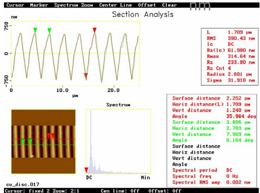
AFM analysis of sinusoidal pattern
