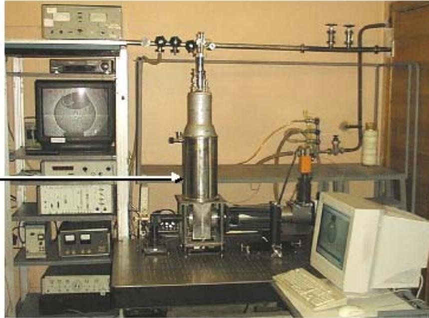
**Experimental facility for cryogenic layering study**
