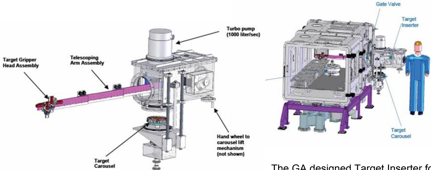
The GA designed Target Inserter for use on Gemini and LIBRA experiments
