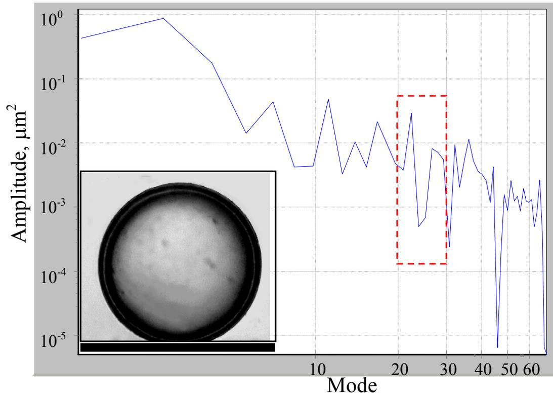
*Fig.3. The results of the FST – layering: fourier-spectrum of bright band shows that layer roughness does not exceed  $0.15 \mu\text{m}$  for modes 20-30*
