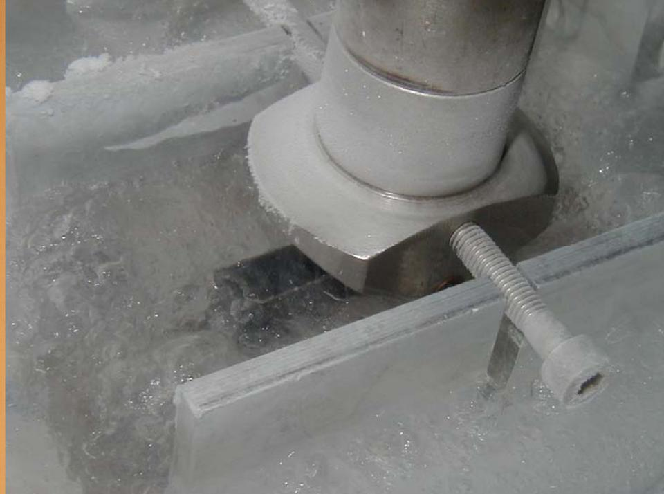
Short beam shear testing at 77K
