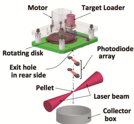
FIG. 1: Pellet injection system.
