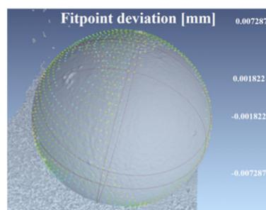
**Figure 3.** X-ray CT scan of ICF shell showing deviation ( $\pm$ 7 $\mu\text{m}$ ) around mean dia. of 1.4mm,  $\rightarrow$   $\sim$ 99% sphericity.
