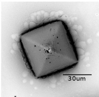
Figure 1: Two-photon-polymerisation produced pyramid with a base length of 37µm.
