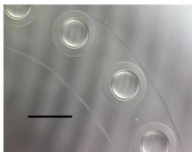
**Figure 1.** TMPTA shells centralising within a fluoropolymer UV photo-microreactor (bar=1000 $\mu\text{m}$ ).
