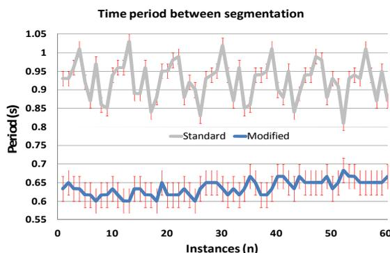
Figure 2 - Two 1ml SGE gastight syringes are used to deliver mineral oil and water into a microfluidic configuration where segmented flow occurs. The time period between the segmentation is extracted from video footage. Flow rate of each fluid is 7.91ml/h.
