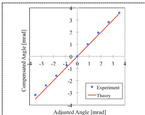
**Figure 2.** Compensation of a PC beam by a PC mirror.
