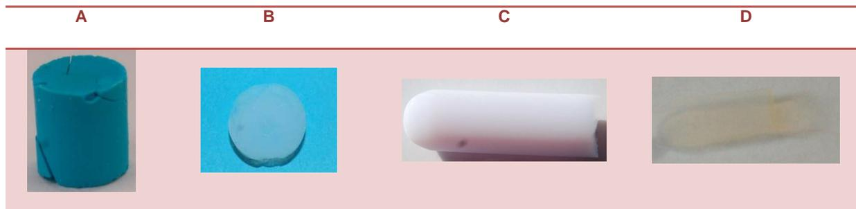
Figure 1: Photographs of copper-based aerogel (A) and lanthanide aerogels: (B) Yb<sub>2</sub>O<sub>3</sub>, (C) Nd<sub>2</sub>O<sub>3</sub>, (D) Tb<sub>2</sub>O<sub>3</sub>.
