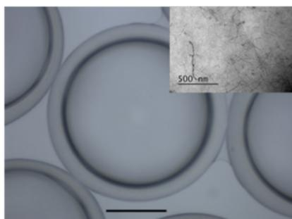
**Figure 2.** Photo-cured TMPTA shells with a concentricity of 99.63%. (bar=500 $\mu\text{m}$ ). Insert shows distribution of CNTs.
