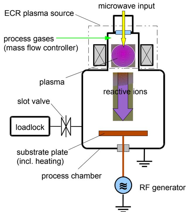
Figure 1: Schematic illustration of PE-CVD
