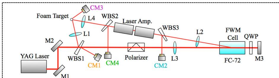
**Figure 1.** Experimental setup for a PC beam compensation.
