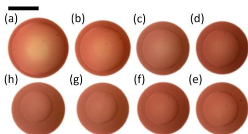
Figure 1 - Images depict individual static compound emulsions, which are suspended in mineral oil. The diameter and wall thickness can be varied, depending on the flow rates into the configuration. Here the independent variable is the outer TMPTA flow. Scale bar is 1mm. Flow rates (ml/h); Water solution= 1.5, TMPTA= a) 0.5, b) 1.0, c) 1.5, d) 2.0, e) 2.5, f) 3.0, g) 3.5, h) 4.0, Mineral oil= 24.0.
