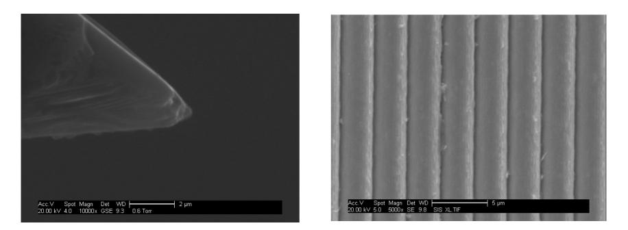
ESEM micrograph of diamond tool showing 'chipping' and wear of the tool tip after cutting 78Km (approximately 3h). A tool under these conditions cannot generate the required profile.
