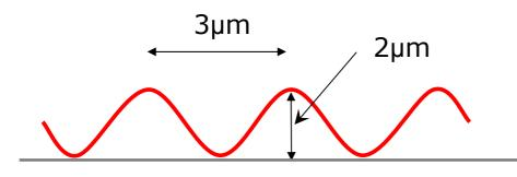
A sinusoidal pattern extending from the edge of an Oxygen-Free High Conductivity Copper disk 13mm inwards. Roughness requirement: 25nm RMS
