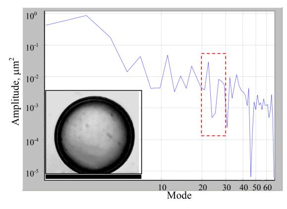
Fig.3. The results of the FST – layering: fourier-spectrum of bright band shows that layer roughness does not exceed 0.15  $\mu$ m for modes 20-30
