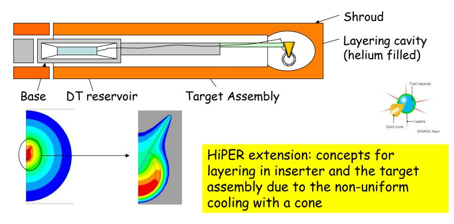
Numerical simulation have to be done to reach the layer shape for fast ignition
