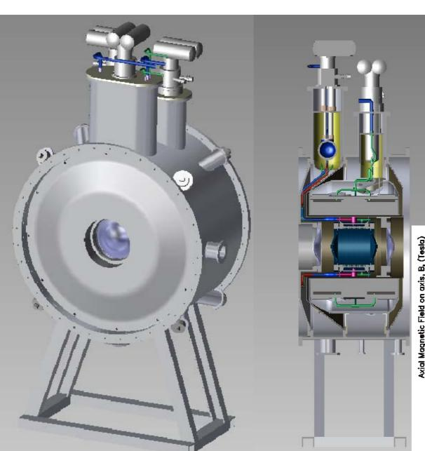
AFC Module for MICE – being produced with Oxford University for the MICE experiment
