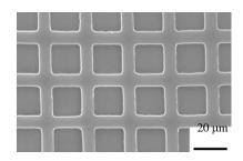
Figure 1: SEM image of microstructures fabricated by EUV irradiation on a PDMS sheet.
