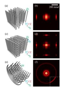
Figure 1: left: laser fabrication of photonic crystal spatial filters; right: different geometries of spatial filters, together with the corresponding light transmission distributions (the far field).
