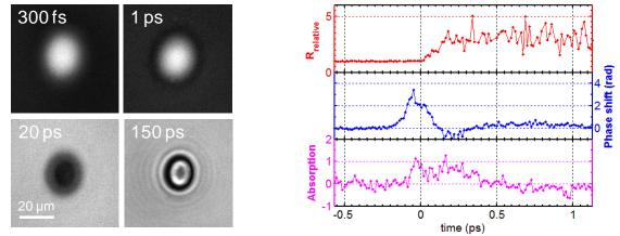
*Figure 1*: (Left) Images of the reflectivity evolution at 800 nm of sapphire excited with a 400 nm, ~80 fs laser pulse above the ablation threshold. (Right) Illustrative example of the simultaneously measured evolution of reflectivity, phase shift, and absorption of fused silica at 400 nm upon excitation with a 800 nm, ~80 fs, laser pulse above the ablation threshold.
