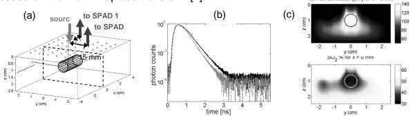
*Fig 1*: Steps of MW/TD reflectance DOT. (a) Drawing of the phantom and scan set-up. (b) Normalized TD measurements of the reference (black continuous line) and the perturbed medium (grey dotted line). (c) Transversal slices of the 3D reconstructed maps of total hemoglobin (HbT) concentration and oxygen saturation (SO<sub>2</sub>) percentage (scale: 50 % threshold of extremum) (Adapted from [3]).
