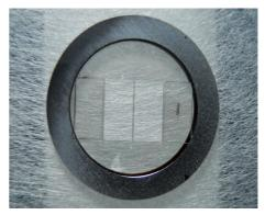
diamond disk, produced by CVD technique, the wire shape has been obtained by cutting the diamond using a FEMTO-EDGE LASER of 1064 nm wavelength.
