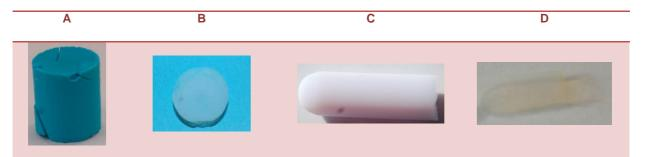
Figure 1: Photographs of copper-based aerogel (A) and lanthanide aerogels: (B)  $Yb_2O_3$ , (C)  $Nd_2O_3$ , (D)  $Tb_2O_3$ .
