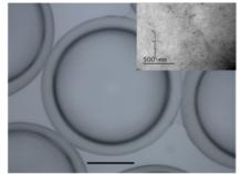
**Figure 2**. Photo-cured TMPTA shells with a concentricity of 99.63%. (bar=500um). Insert shows distribution of CNTs.
