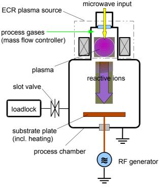
Figure 1: Schematic illustration of PE-CVD
