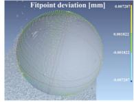
**Figure 3.** X-ray CT scan of ICF shell showing deviation (+/-7um) around mean dia. of 1.4mm, --> ~99% sphericity.
