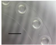
**Figure 1.** TMPTA shells centralising within a fluoropolymer UV photomicroreactor (bar=1000um).
