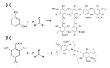
Fig. 1. Scheme of polymerization of the (a) resorcinol-formaldehyde (R-F) gel and (b) Phloroglucinol carboxylic acid-formaldehyde (PC-F) gel.
